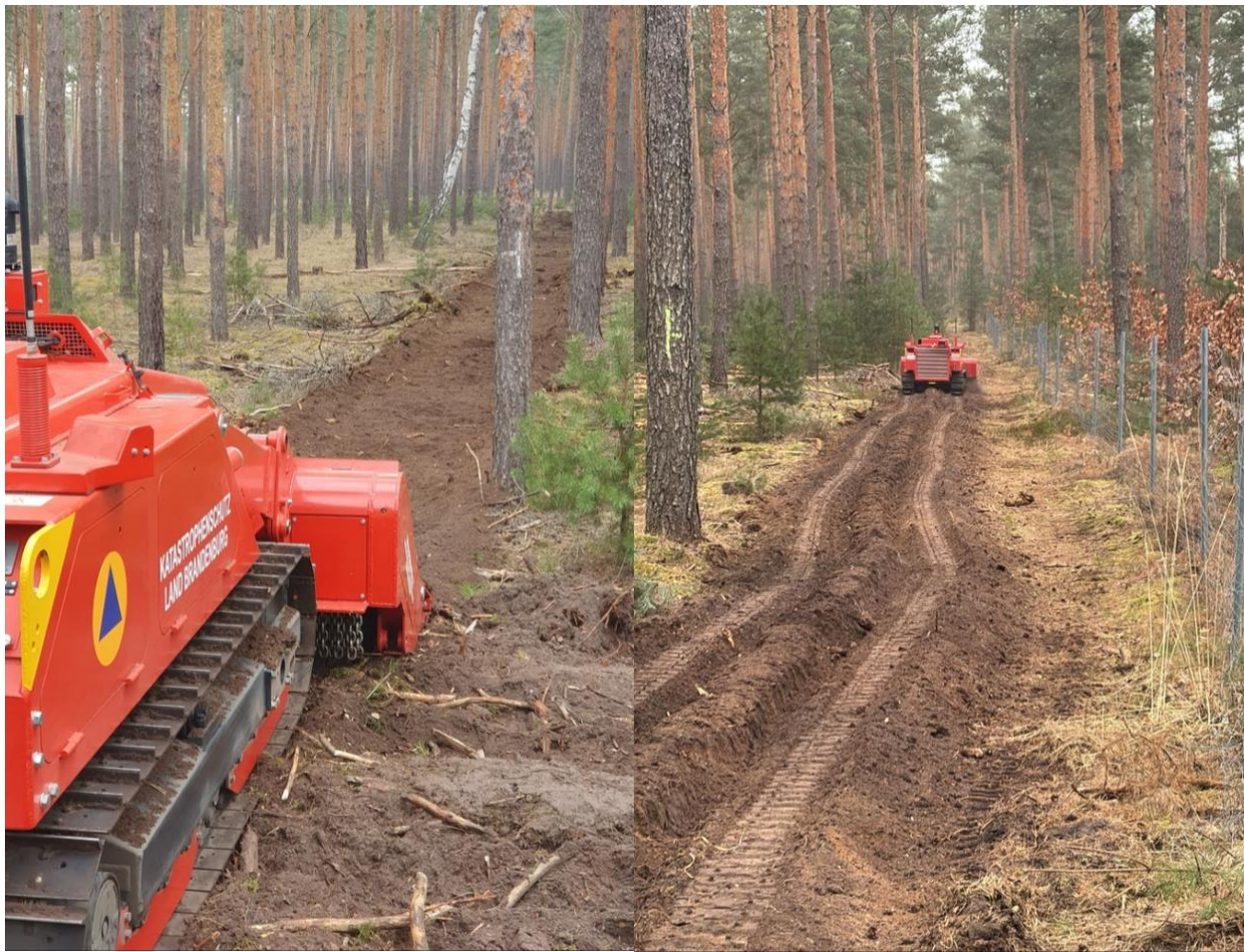
Photos: N. Barth. Preventive establishment of control lines by the MV-4, Brandenburg, 2025.
