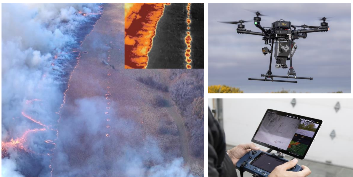
Photos: Drone Amplified. Precise, GPS-guided aerial ignition with Ignis Drone Amplified .
